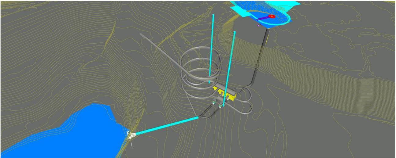
**Figure 1:** Overhead design of the internal structure between the two reservoirs showing the axis spiral decline, intake shaft (far right), cable shaft (middle) and emergency egress (left) and the tailrace tunnel at the bottom.
