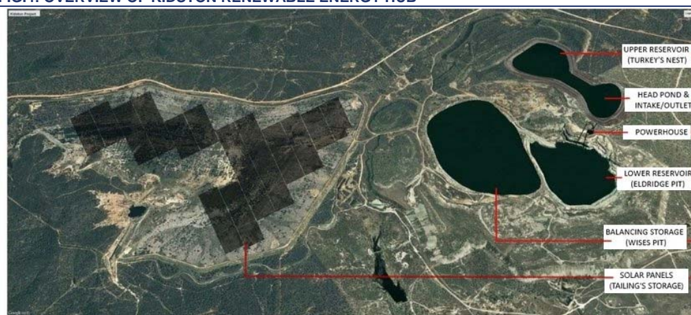
FIG.4: OVERVIEW OF KIDSTON RENEWABLE ENERGY HUB
