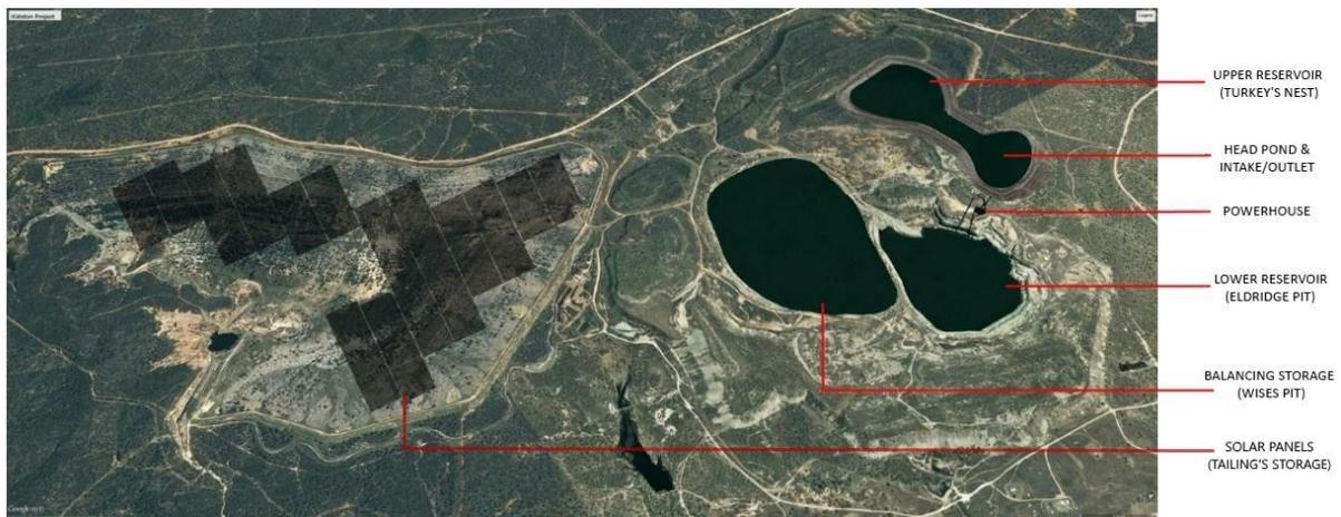
The hub, located in Kidston in Northern Queensland, will comprise three renewable energy projects: a 50 MW solar project (Kidston Solar Project Phase One 50 MW, or KSP1); a 250 MW pumped-storage hydro project (Kidston Pumped Storage Hydro Project, or KPSHP) and an additional 270 MW solar project (Kidston Solar Project Phase Two 270 MW, or KSP2).
