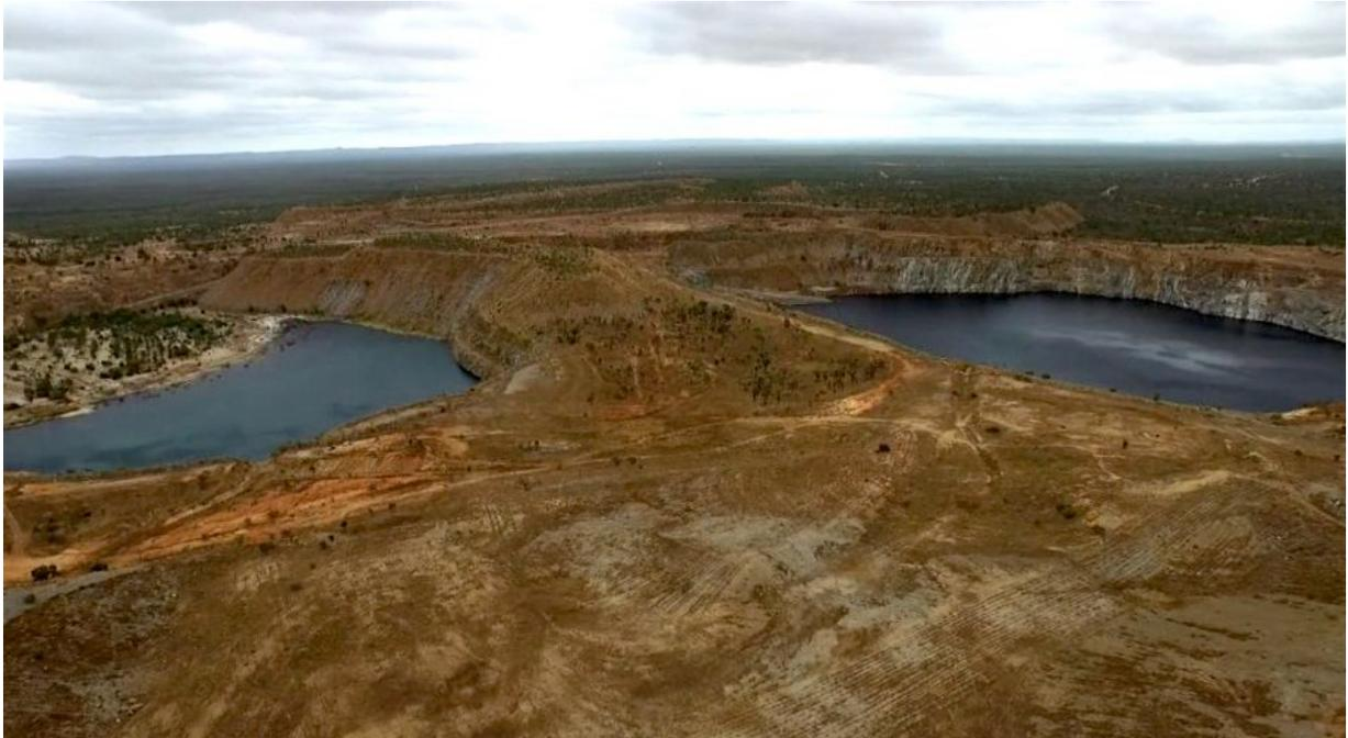
Kidston mine's two large mine pits will be turned into a pumped hydroelectric energy storage (PHES) system. (Image courtesy of [Genex](#))
